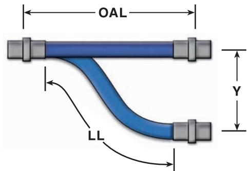
**Note:** Where offset motion "Y" occurs on both sides of hose centerline, the hose live length should be based on total travel, or 2Y. The modified calculation will be:
